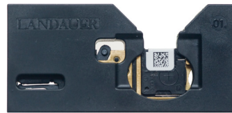
nanoDot carriers slide in and out of the adapter (2D bar code facing front) for read-out in a microStar reader.
