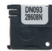
Front of nanoDot carrier with alphanumeric sensitivity code and serial number (DN091=0.91 sensitivity). Either the front or back of the carrier can face toward the radiation source during exposure.
