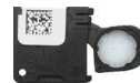
Back of open nanoDot carrier with 2D bar code that includes sensitivity code and serial number.
