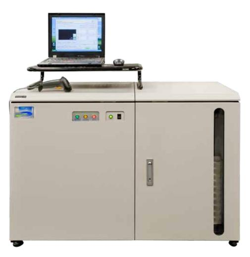
The Auto 500 is designed for heavy, high-speed loads. It uses aluminum oxide  $(AI_2O_3)$  detectors to measure radiation exposure and reads the measurement with optically stimulated luminescence (OSL) technology. These readers are ideal for any radiation assessment application.
